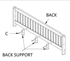
**3)** Attach Back Supports to Back using (1) C Bolt for each Back Support as shown.
