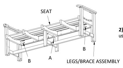
**2)** Attach Seat to Legs/Brace Assembly using (2) A Bolts and (4) B Bolts as shown.
