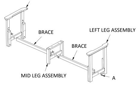
1) Attach Braces to Leg Assemblies using (8) A Bolts.
